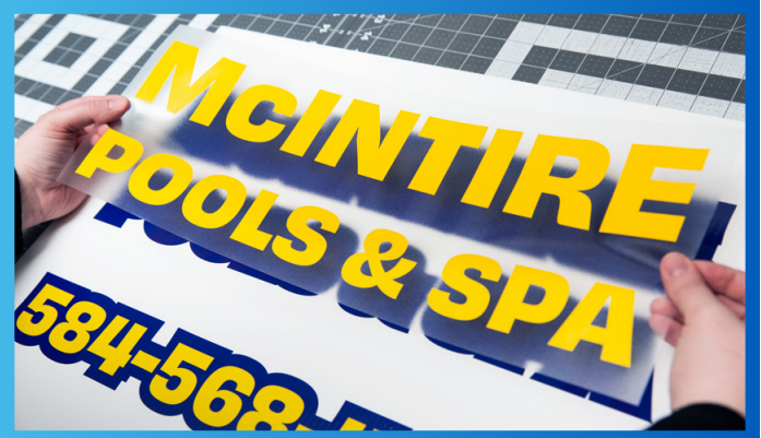
1310 is the best choice for drop shadows, where perfect alignment is critical. Seeing through the tape allows you to be sure you've lined it up just right.
